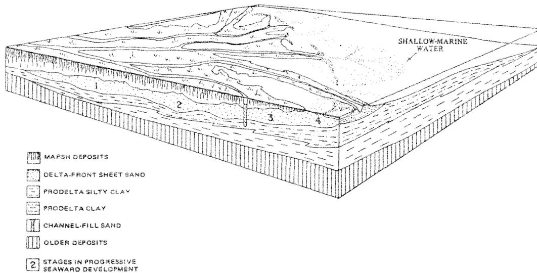
Figure 4. The structure and components of a shallow water delta (from Gould 1970).
